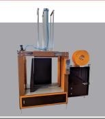
Unwinders: custom made out of heavy duty steel according to width of fabric as discussed with the customer. Popular sizes include : 6, 9, 10, & 12 feet.
